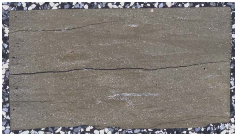
T-201 RC-8 67'5"-69'6" E3M-011.jpg/XPL/FOV = 27 x 46 mm LIMESTONE showing typical appearance.
