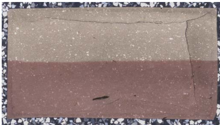
T-204 52'10"-55' E3M-015.jpg/XPL/FOV = 27 x 46 mm LIMESTONE showing typical appearance.
