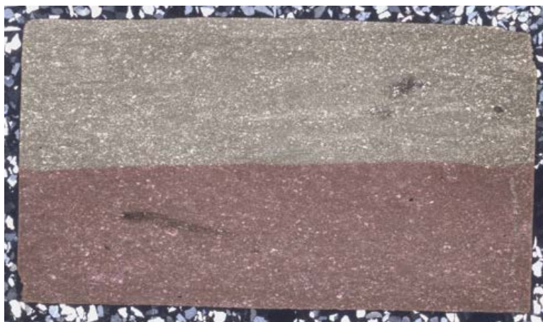
P-102 26'-28'4" E3M-001.jpg/XPL/FOV = 27 x 46 mm LIMESTONE showing typical appearance.
