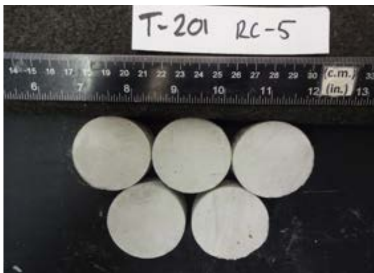
Sample before testing (specimen would fail if more than one drill location was used)
