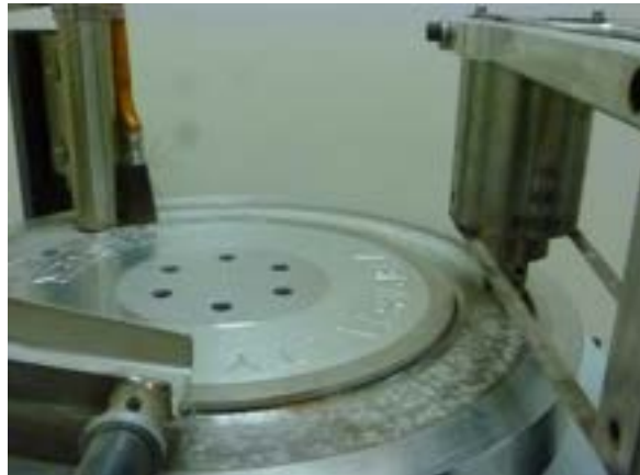
Closeup of Abrasivity machine with sample
