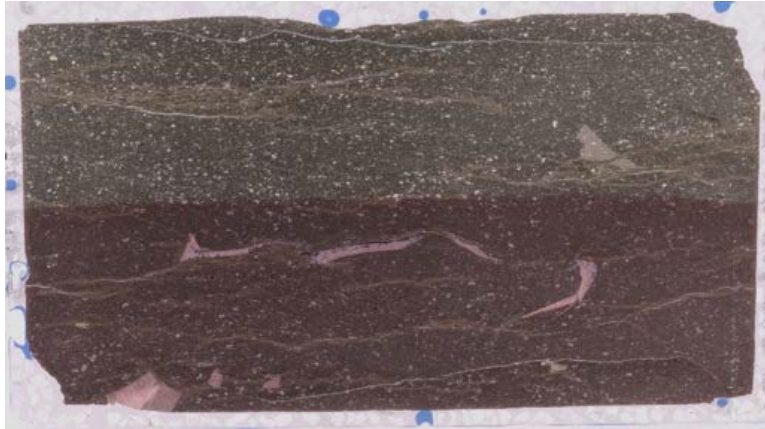
TS-202 RC-6/7 60'-64'1" E3M-032.jpg/PPL/FOV = 27 x 46 mm LIMESTONE showing typical appearance.
