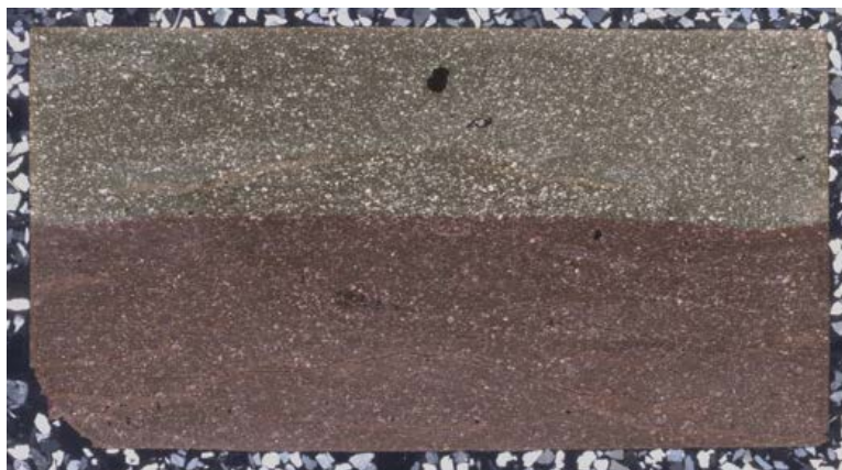
TS-104 RC-7 60'-63'5" E3M-027.jpg/XPL/FOV = 27 x 46 mm LIMESTONE showing typical appearance.
