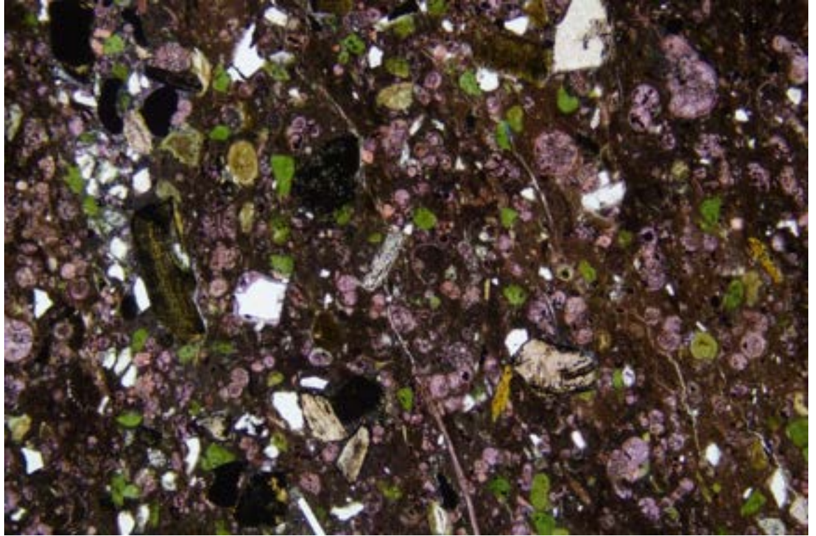
T-201 RC-7 63'10"-65' E3M-042.jpg/PPL/FOV = 1.85 x 2.69 mm CLAYSTONE showing typical appearance.
