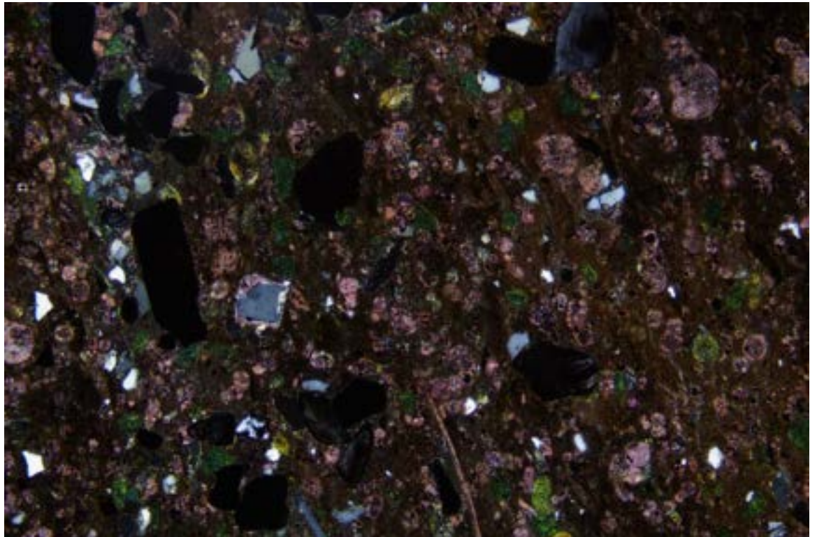
T-201 RC-7 63'10"-65' E3M-041.jpg/XPL/FOV = 1.85 x 2.69 mm CLAYSTONE showing typical appearance.
