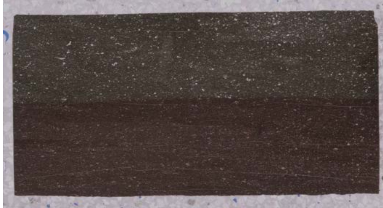
TS-104 RC-5 53'3" E3M-026.jpg/PPL/FOV = 27 x 46 mm LIMESTONE showing typical appearance.
