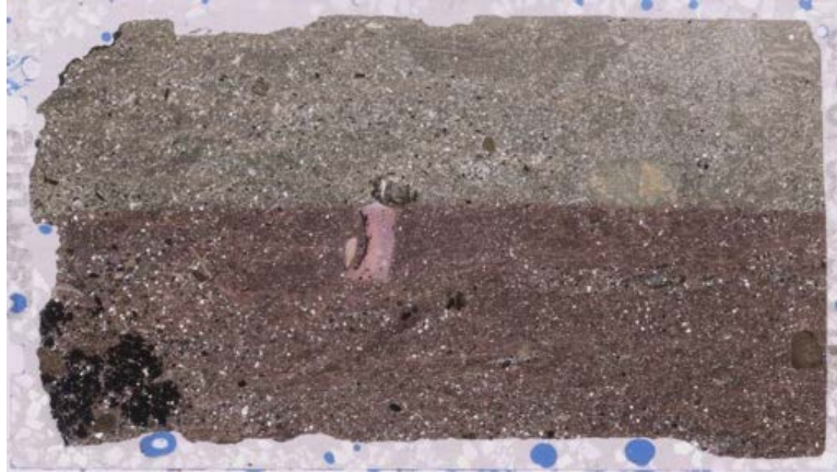
T-201 RC-7 63'10"-65' E3M-010.jpg/PPL/FOV = 27 x 46 mm CLAYSTONE showing typical appearance.
