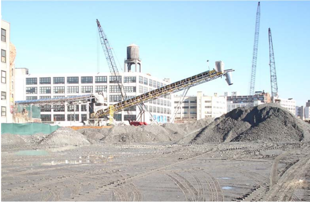
FIGURE 3-2. RADIAL STACKER BELT CONVEYOR LOADING ONTO STOCKPILES IN SUNNYSIDE YARD (EAST SIDE ACCESS PROJECT)
