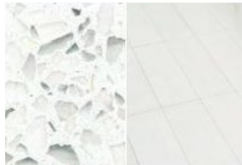
FLOOR FINISH 02 INTERIOR FLOORING ACCENT Material: Terrazzo Color: White (Matrix aggregate TBD) Surface Finish: Smooth, slip-resistant
