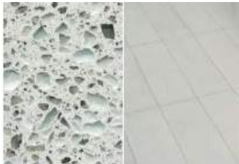
FLOOR FINISH 01 TYPICAL INTERIOR FLOORING Material: Terrazzo Color: Grey (Matrix aggregate TBD) Surface Finish: Smooth, slip-resistant Precast stair treads & risers in same finish with cast-in metal tread abrasives. BOD Product: Wasau precast terrazzo
