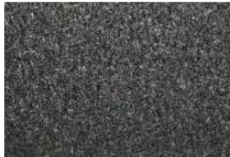
FLOOR FINISH 06 TYPICAL EXTERIOR FLOORING / STREET LEVEL ENTRY FLOORING Material: Granite Color: Grey Surface Finish: TBD Filed Tile Size: TBD
