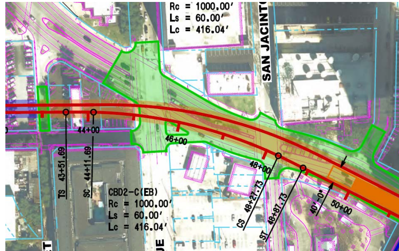
Figure 5-1 Layout of the West Portal and Cut-and-Cover Excavation (as of 8/12/2019)
