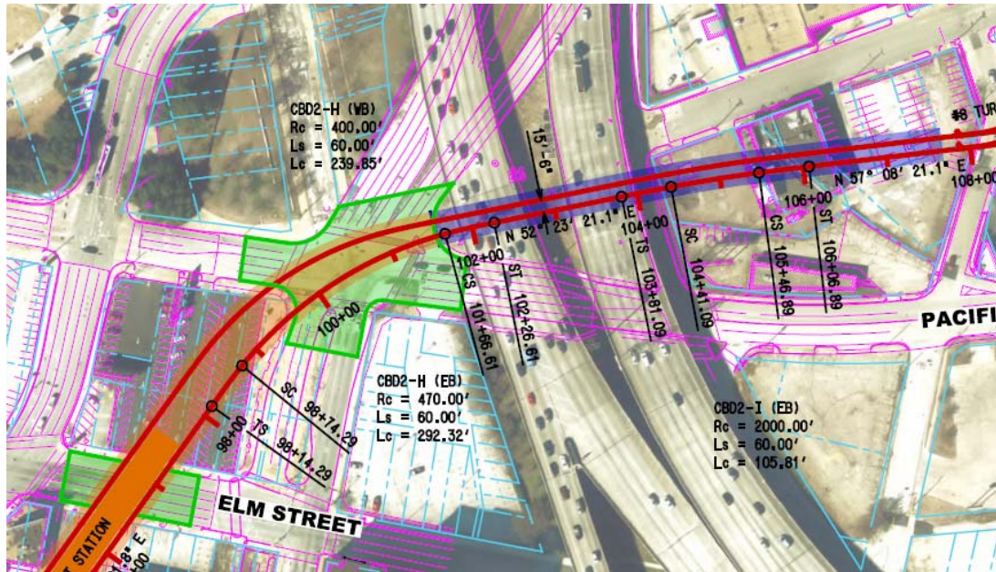
Figure 5-14 Layout of the East Portal and Cut-and-Cover
