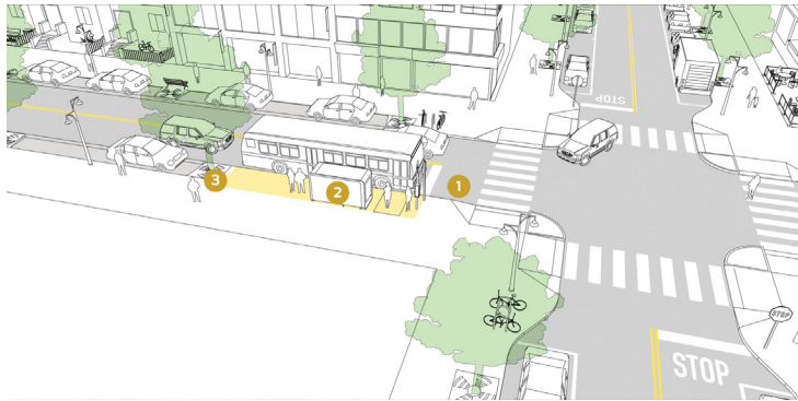
Figure 9: Bus Bulb Example from NACTO
